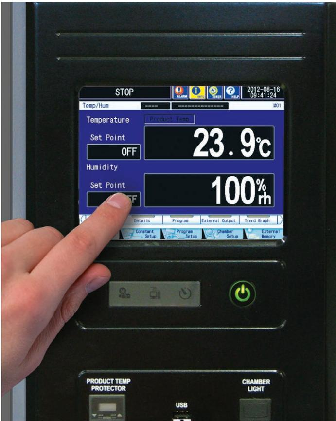
The door-mounted console includes the P-300 programmer, USB port, product temperature protector, and chamber light (option).
