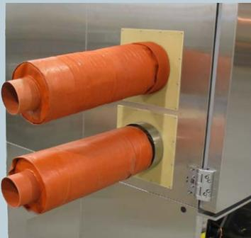
Allows conditioning of remotely-located equipment that cannot be placed inside the chamber.
