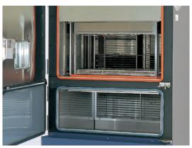
TSD-101-W Test areas (Top: hot chamber Bottom: cold chamber)
